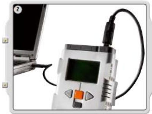
Connect the PC and the NXT with the USB cable.
